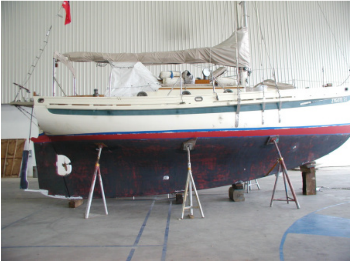
Image 4. 2005. Inside the paint shed at Wavemaster, on Langkawi, Malaysia: Four keel blocks and six tripod stands (not chained together athwartships!). Block 1 is under Bulkhead 2. The LCG is midway between Blocks 2 and 3. Block 4 is under a void filled with mish-mash. Tripod stands 1, 2, and 3 are at Bulkheads 3, 4, and 6.
