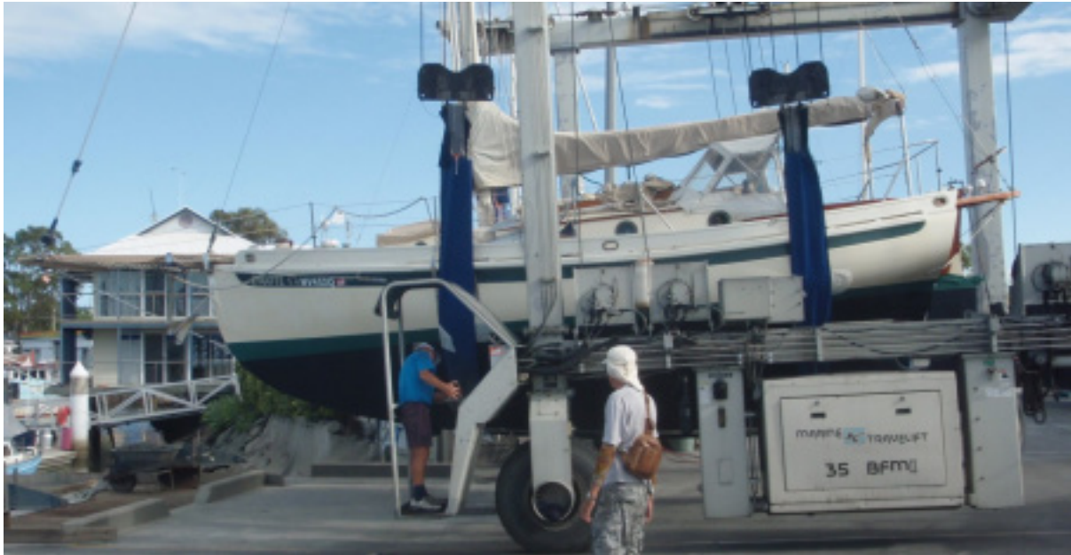
Image 1. 2011, at Scarborough Marina, QLD. Steve Kviklys driving a 35 tonne Marine Travelift and preparing to re-launch Zygote . Forward sling at Bulkhead 3 between Chainplates 1 and 2; Aft sling at Bulkhead 6.
