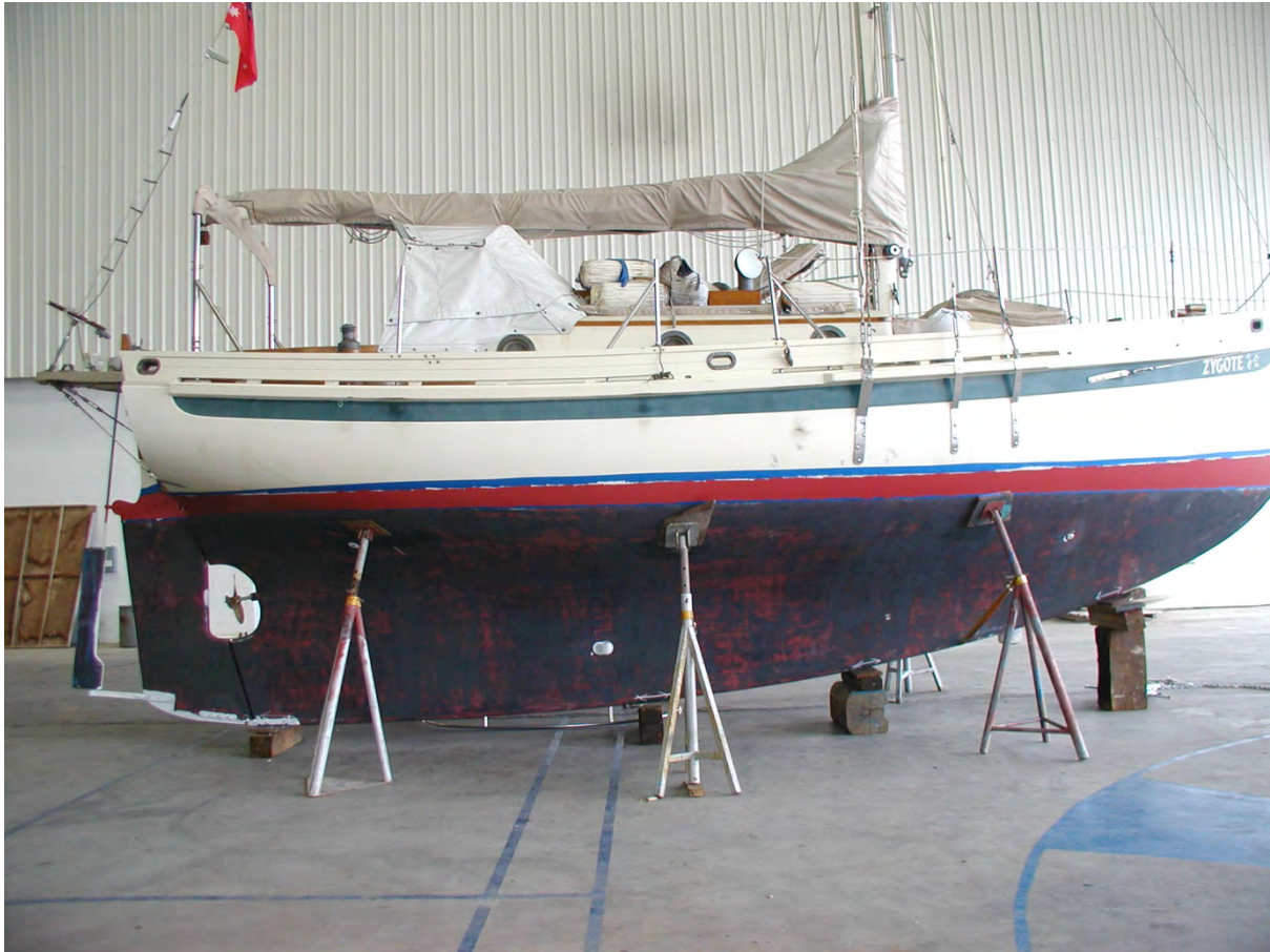
Image 5. 2005. Inside the paint shed at Wavemaster, Langkawi, Malaysia: Four keel blocks and six tripod stands (not chained together athwartships!). Block 1 is under Bulkhead 2. The LCG is midway between Blocks 2 and 3. Block 4 is under a void filled with mish-mash. Tripod stands 1, 2, and 3 are at Bulkheads 3, 4, and 6.
