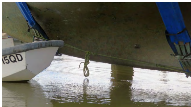
Image 1. 2022 lift at Scarborough Marina, with slings lashed together.
