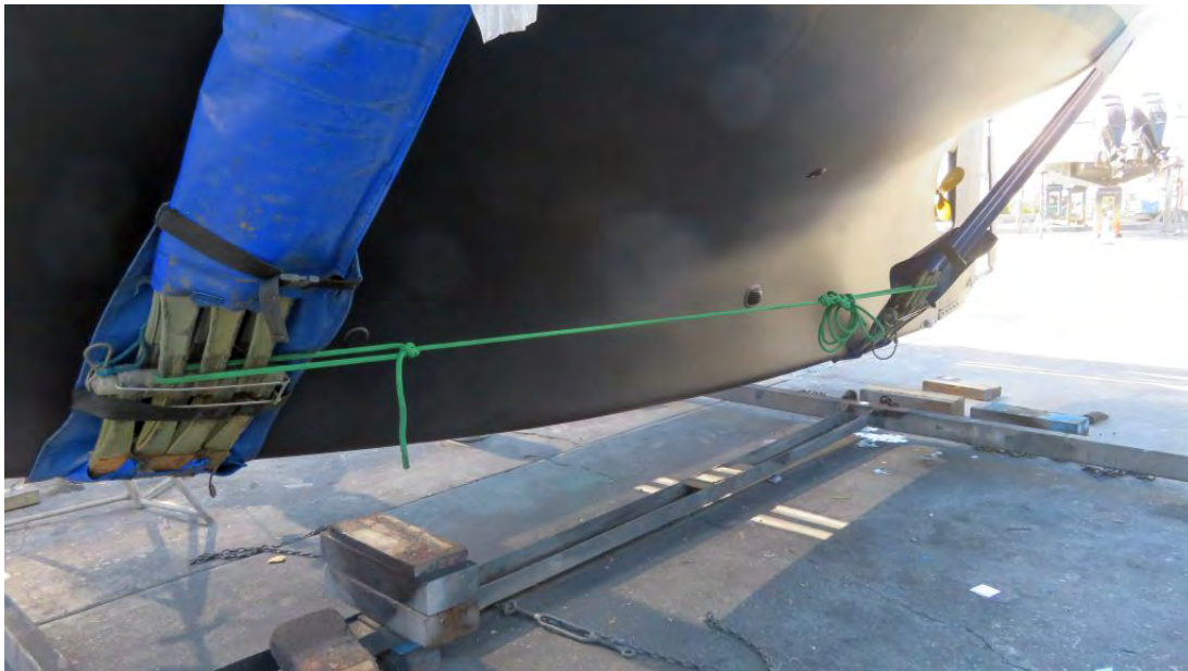
Image 7. 2022. Lashing between fore and aft slings at Scarborough Marina, QLD, just prior to relaunch.
