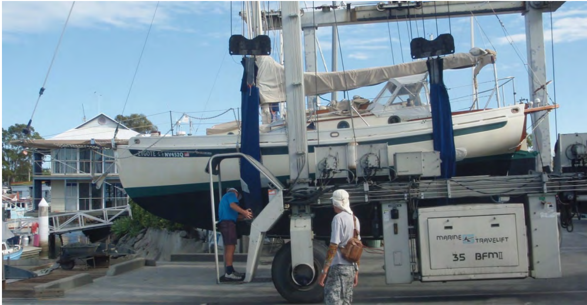
Image 2. 2011, at Scarborough Marina, QLD. Steve Kviklys driving a 35 tonne Marine Travelift and preparing to re-launch Zygote. Forward sling at Bulkhead 3 between Chainplates 1 and 2; Aft sling at Bulkhead 6.
