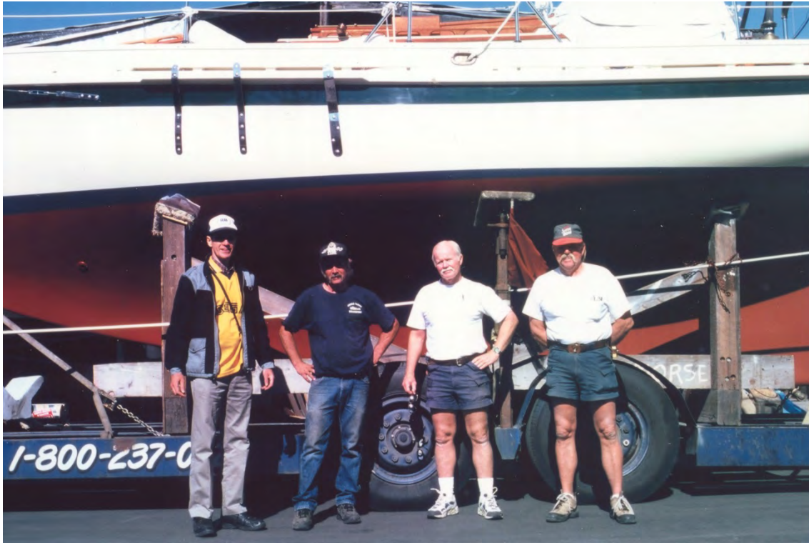
Image 4. 2000. Sam L. Morse Co. boatyard at Costa Mesa, CA, with Denny of Joule Yacht Transport, and master shipwrights Dick McComb and Tommie Whisler of Sam L Morse Co.: 4-leg box cradle with two jack stands (for extra stability on the lowboy towed by a Freightliner, which reached a top speed of 38 mph without the boat shifting position) and strap ties. The box cradle has its legs close to Bulkheads 3 and 6. The jack stands are at Bulkhead 4. The cradle legs were 6 x 6 inches; the legs were 12 ft 6 inches apart, centre to-centre.
