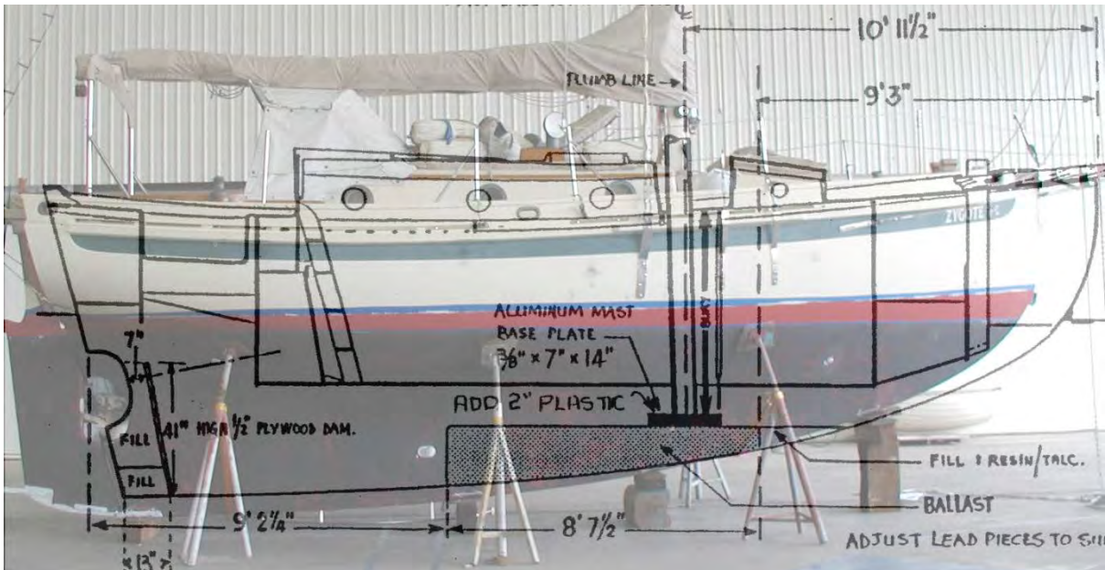
Image 6. Boat photo with overlay of structural profile (note unavoidable lack of registration between the profile drawing in isometric projection and the photographic image in perspective).
