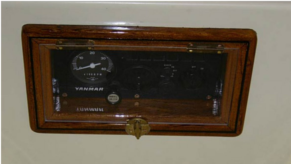
Figure 3: Installed recessed engine control panel.
